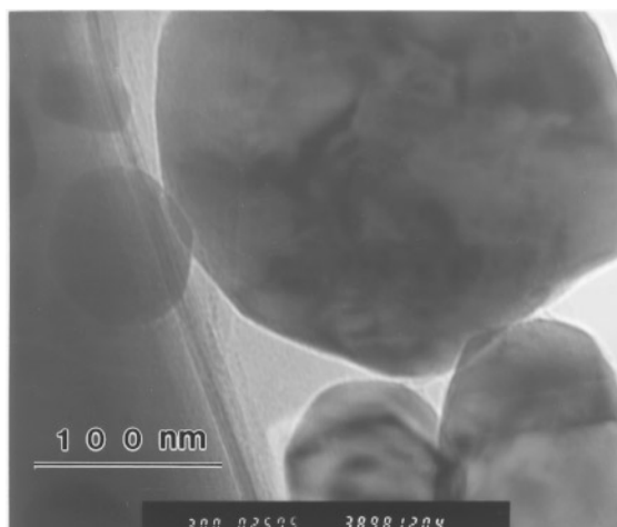
Figure 1. Bright field transmission electron microscope (TEM) photograph of a typical sample of palladium nanoparticle encapsulated in graphite host. The picture was taken with a Hitachi H-9000 TEM operated at 300 kV.
